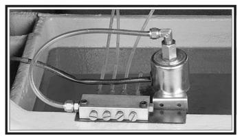
Figure 44. Lubrication pump and reservoir.
